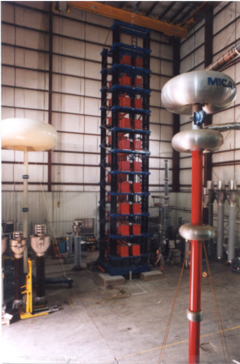
20 Stage – 3,600,000 kV Impulse Generator
